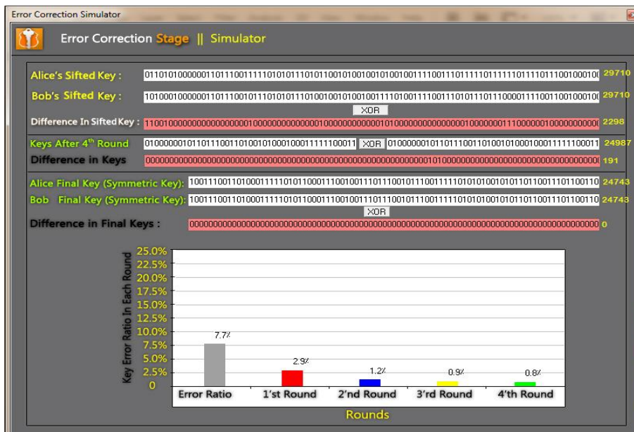
Figure (6) – shows the error correction simulator, the error ratio between the two key is 7.7%, the Sifted Key length is 29710 bits and the Number of photons being sent is 60000 photons.
